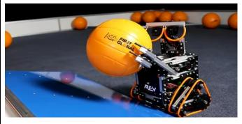
[4] The Moroccan team created a robot that can move on unstable surfaces, such as beach sands. The robot was also able to carry 15 to 20 waste items, such as candy wrapping, soda cans, and plastic boxes. Finally, the Moroccan invention could lift the items up to 70 cm high and dispose of them in a trash bin.
